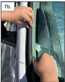
8. The finished project should appear as shown. You will then be able to run your wiring through by gently pulling the rubber lip up on the side and sliding the wiring into place.
